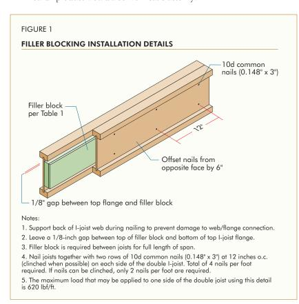
equal the distance between the flanges of the I-joist minus 1/8 inch. This gap is placed between the filler block and the top flange. The reason for the gap is to prevent the inadvertent use of a slightly oversized block. Forcing such a block to fit between the flanges of an I-joist could damage the joist to the point where it may not function as designed.
