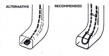
Figure 22. Cable in "end of run" downspouts
