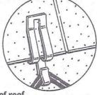
Figure 12. Attaching clips to shingles at top of triangles
