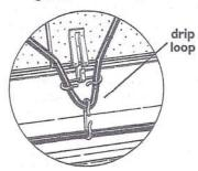
Figure 13. Attaching clips to shingles at edge of roof with gutters
