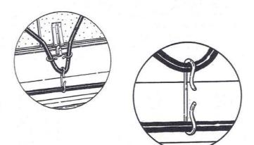
Figure 19. Attaching clips in gutters
