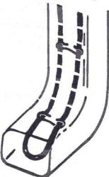
Figure 20b. Double run of cable in gutter-only applications (gutters without gutter spikes)
