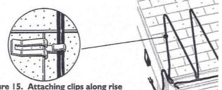
Figure 15. Attaching clips along rise of larger triangles
