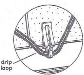
Figure 14. Attaching clips to shingles at edge of roof without gutters RC Owner's Manual
