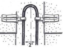
Figure 17. Attaching clips in valleys RC Owner's Manual <u>Routing the cable along the gutter using cable spacers.</u> This section describes how to route the cable along the gutter using spacers.
