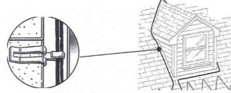
Figure 16. Attaching clips around dormers
