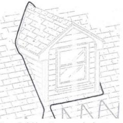
Figure 7. Cable pattern around a dormer
