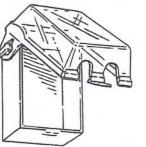
Is within 6 feet of the cable starting point on the roof. [Refer to Planning Your Cable Arrangement on pages 10 – 13.] The power cord of the cable is 6 feet long, and the remainder of the cable is heated. Choosing a receptacle that is within 6 feet of the start point will make sure that the heated portion of the cable is entirely on the roof. This will also avoid contact by persons or equipment (such as yard tools) that can move or damage the cable.
