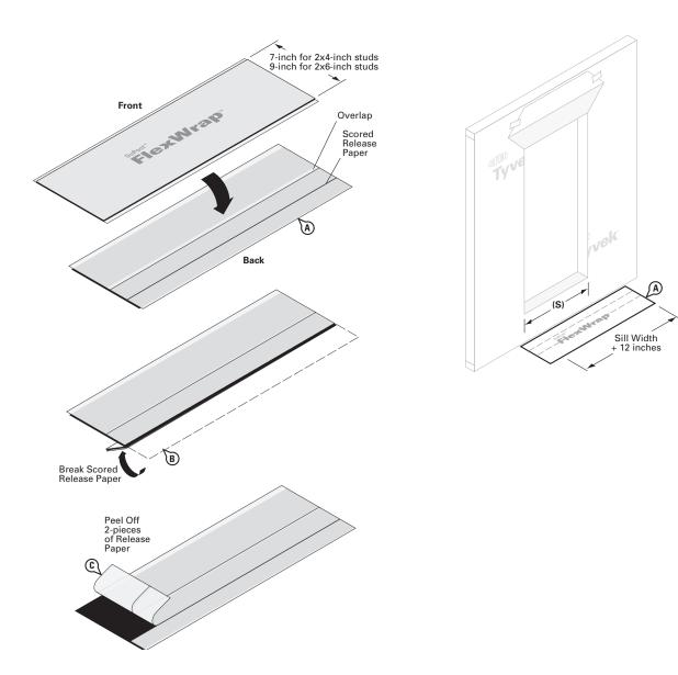
A. Install the sill flashing as indicated leaving the 1" of DuPont<sup>™</sup> FlexWrap<sup>™</sup> with release paper extending it past the door threshold on the inside. When the 1" of release paper is removed, there should be 3/4" of flashing to form the back dam.
