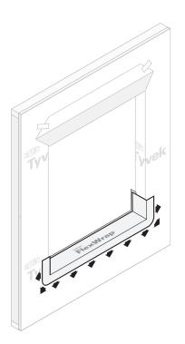
A. SECURE EDGES OF DUPONT<sup>™</sup> FLEXWRAP<sup>™</sup> WITH DUPONT RECOMMENDED FASTENERS along the bottom outer edge of the DuPont<sup>™</sup> FlexWrap<sup>™</sup> at fanned corners.
