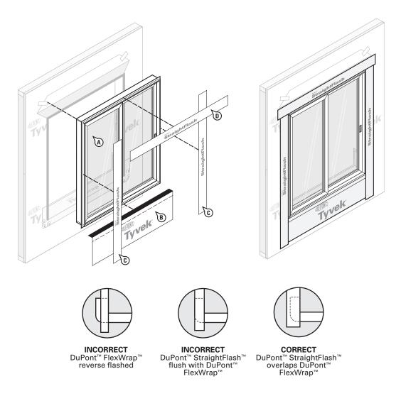
**NOTE:** Do not reverse shingle. DuPont<sup>™</sup> StraightFlash<sup>™</sup> must overlap DuPont<sup>™</sup> FlexWrap<sup>™</sup> and adhere to the substrate.
