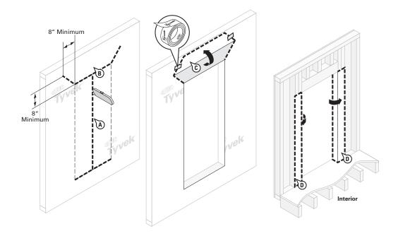
Preparation of sill flashing:
