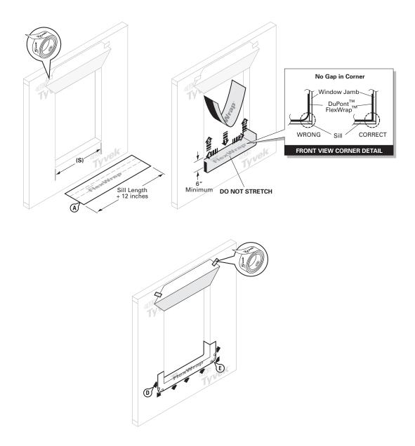
A. Apply continuous bead of DuPont<sup>™</sup> Weatherization Sealant at the window head and jambs to wall or back side of window mounting flange. DO NOT APPLY CONTINUOUS SEALANT BEAD ACROSS BOTTOM SILL to allow for drainage.
