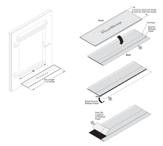
A. Install the sill flashing as indicated leaving the 1" of DuPont<sup>™</sup> FlexWrap<sup>™</sup> with release paper extending it past the door threshold on the inside. When the 1" of release paper is removed, there should be 3/4" of flashing to form the back dam. Optional: Some flooring cannot accomodate a back dam. In that case, fold the 1" back dam on top of DuPont<sup>™</sup> FlexWrap<sup>™</sup> in the sill. Door will be installed on top of the 1" fold to create a back dam.
