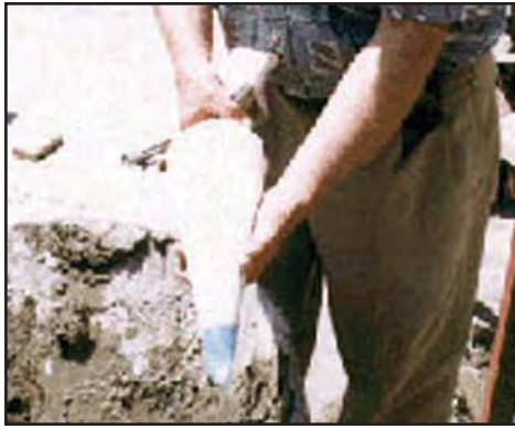
2. Holding the top of the bag, twist approximately one complete revolution or more to take up slack.
