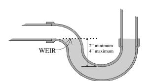
The weir of a p-trap <u>must</u> be below the top of the opening in the fitting that connects it to it's vent.
