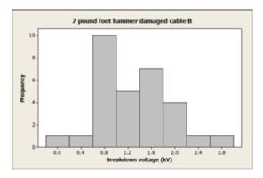
100% of cable B samples with 5 pound foot hammer damage failed 6kV breakdown voltage test 100% of cable B samples with 7 pound foot hammer damage failed 6kV breakdown voltage test
