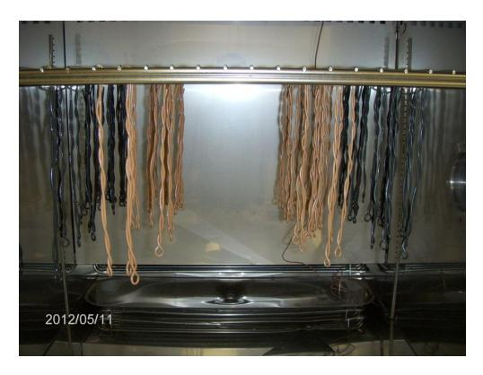
Figure 35 - Black and white NM cable conductors in the test chamber for thermal aging
