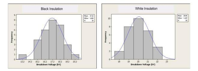
Figure 14 - Cable A breakdown voltage distribution
