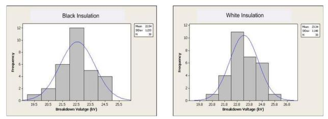
Figure 18 - Cable E breakdown voltage distribution
