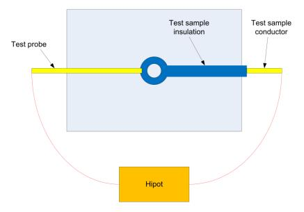
Figure 12 - Cross-section of the Teflon fixture for the NM cable breakdown voltage test
