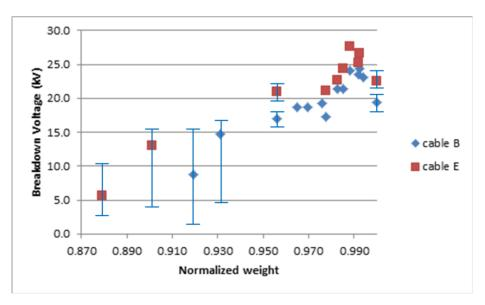
Figure 40 - Breakdown voltage and normalized insulation weight from samples aged at 120 °C, 135°C and 150°C. The error bars indicate the range of the test data.
