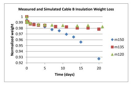
Figure 38 – Cable B insulation weight loss under different temperatures. m150 is the data at  $150^{\circ}$ C, m135 is the data at  $135^{\circ}$ C, and m120 is the data at  $120^{\circ}$ C.
