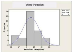
Figure 15 - Cable B breakdown voltage distribution
