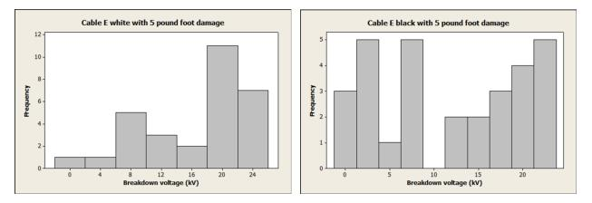
Figure 30 - Breakdown voltage distribution of hammer-damaged NM cable insulation
