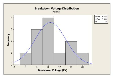
Figure 41 – Cable B insulation breakdown voltage distribution after aged at 150 <sup>o</sup>C for 29 days
