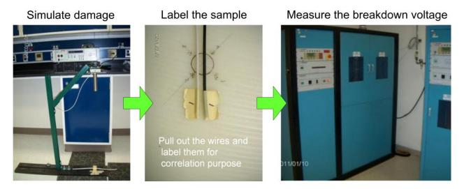
Figure 28 - Step-by-step procedure for damage to NM cable through direct hammer hit
