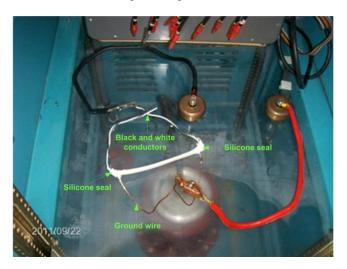
Figure 42 – Setup for the breakdown voltage test for intact NM Cable
