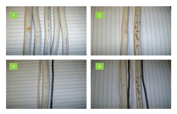
Figure 24 - Overdriven NM cable samples
