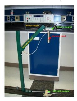
Figure 27 - Hammer impact simulator
