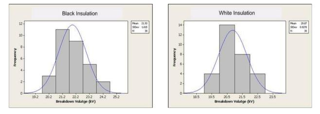
Figure 17 - Cable D breakdown voltage distribution
