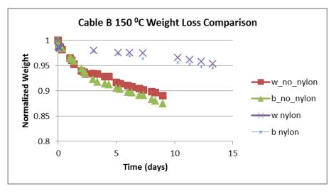
Figure 36 Comparison of Cable B insulation aging with and without nylon layer
