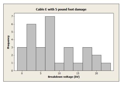
Figure 31 - Breakdown voltage distribution for combined black and white insulation (Example using Cable E data from a 5 ft-lb hammer blow)
