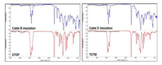
Figure 10 - FTIR spectrum for Cable B and Cable E insulation
