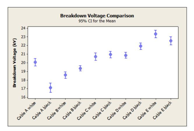
Figure 13 - Average breakdown voltage comparison
