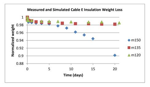
Figure 39 – Cable E insulation weight loss under different temperatures. m150 is the data at  $150^{\circ}$ C, m135 is the data at  $135^{\circ}$ C, and m120 is the data at  $120^{\circ}$ C.
