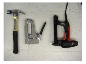
Figure 2 - NM cable installation tools
