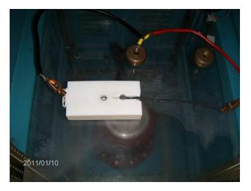
Figure 11 - Fixture for the NM cable breakdown voltage test
