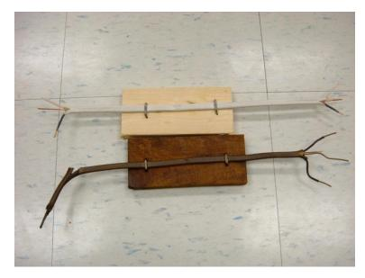
Figure 45 – Hammer-damaged and aged NM cable samples for the UL1449 test.
