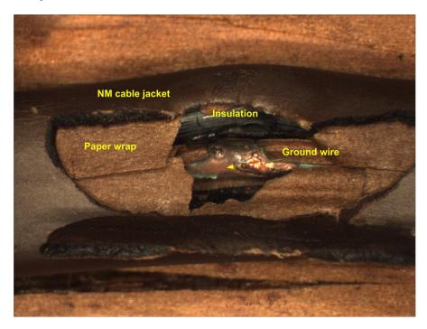
Figure 48 - Arcing area of damaged NM cable
