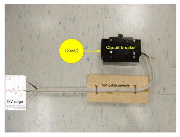
Figure 46 – NM cable voltage surge test schematic.
