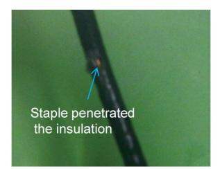
Figure 20 - NM cable damaged by misaligned staple
