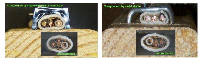
Figure 22 - NM cable compressed by a staple with plastic insulation
