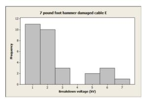
About 37% of cable E samples with 5 pound foot hammer damage failed 6kV breakdown voltage test. More than 90% of cable E samples with 7 pound foot hammer damage failed 6kV breakdown voltage test.
