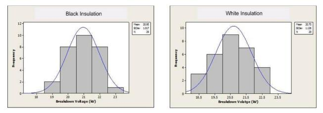
Figure 16 - Cable C breakdown voltage distribution
