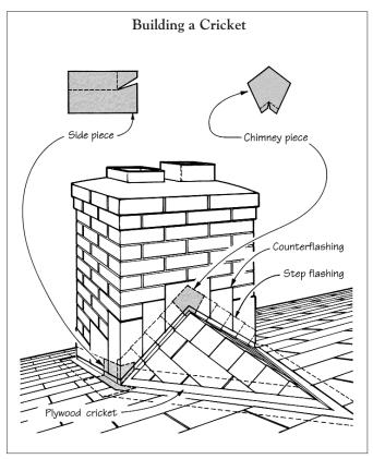
**Figure 3.** You can build the cricket from plywood and cover it with shingles or metal flashing (for a small chimney). The joint at the cricket is step-flashed and counterflashed like the rest of the chimney.
