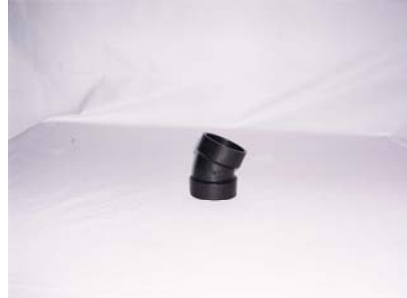
1/16 bend– 22 1/2 degree bend. This fitting is used to offset drain and vent pipe. Can be used in any position.
