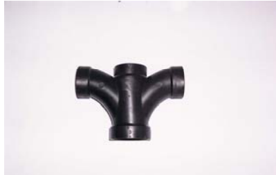
Double Fixture fitting. Used for connecting back to back fixtures with fixture rim heights at same level or under floor for back to back toilets. This is not a double san tee.
