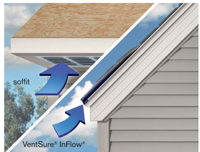
Figure 22 - Types of intake ventilation
