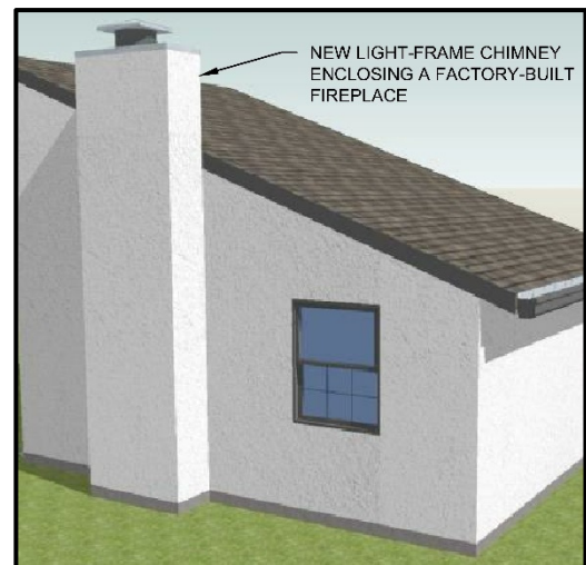
Figure 10: Replacement of entire firebox and chimney with light-frame construction.
