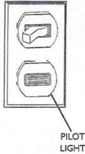
Figure 1a. ON/OFF switch with indicator (pilot light)
