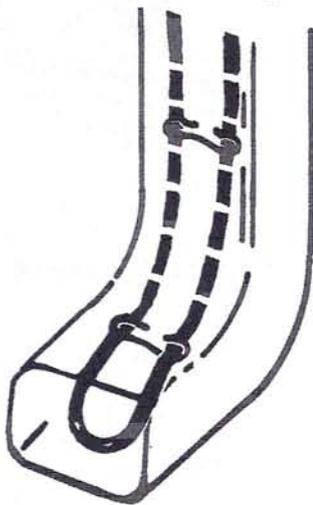
Figure 21. Double cable run in “along run” downspouts
