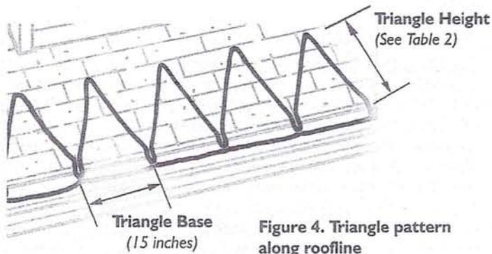
**Figure 4. Triangle pattern along roofline**
