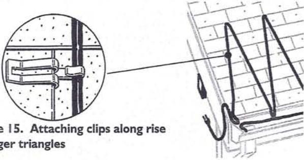
Figure 15. Attaching clips along rise of larger triangles
