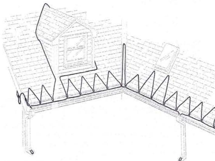
Figure 3. Typical pattern along roofline and in gutters/downspouts
