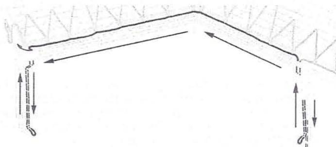
Figure 8. Cable routed back along the roofline in the gutter and downspouts
