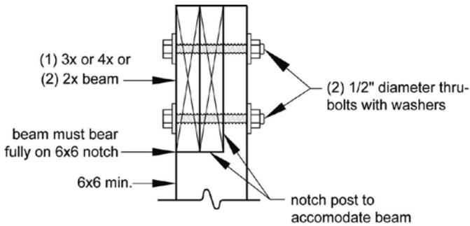
**Figure 9. Prohibited Post-to-Beam Attachment Condition**
