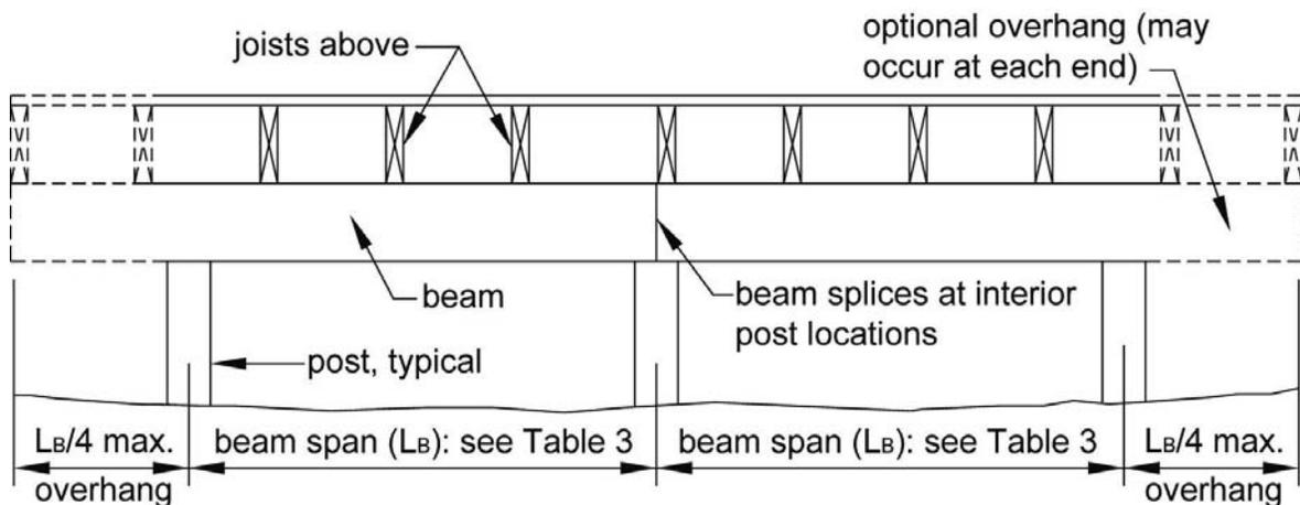
**Figure 4. Beam Assembly Details**
