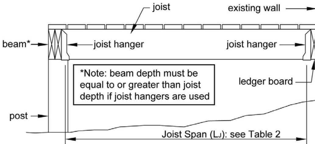
Figure 2. Joist Span – Free Standing Deck
