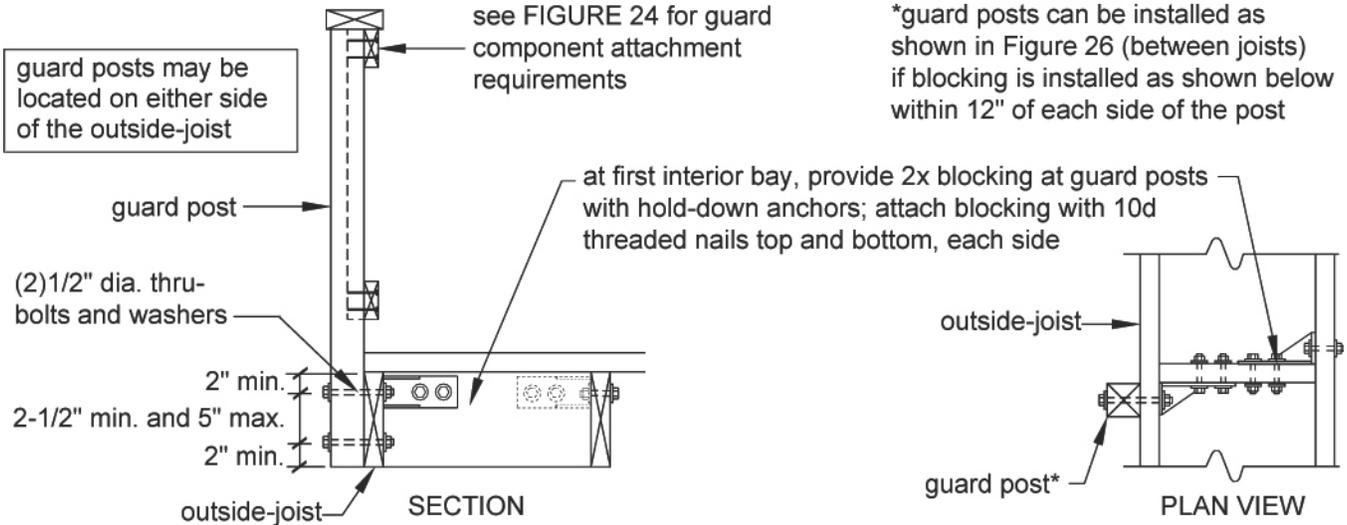
**Figure 26. Guard Post to Rim Joist Example**
