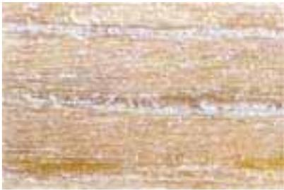
The final slide showed weathered cedar brightened with Bio-Wash WoodWash restorer. The citric acid used in the cleaner gets rid of the dead wood fibers but does not effect the natural bonding agent in the wood.
