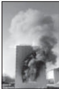
2 Story EIFS Fire Test
