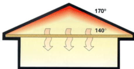
The principal source of attic heat is solar heat gain from direct sunlight on the roof. Even on a cloudy day there is an appreciable amount of heat transmitted to the roof. This solar heat is transmitted through the roof material and, in turn, is radiated to the attic floor -- or to the top surface of the ceiling insulation. This surface becomes heated, and the attic air in contact with the underside of the roof and the top of the insulating material also becomes heated.
