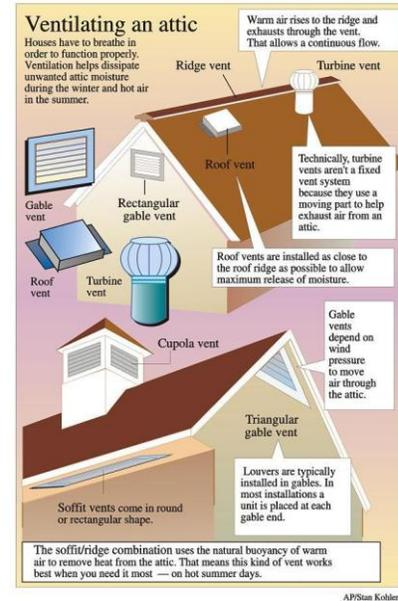
One of the critical aspects of a roof system's durability is the ventilation of the attic or space below the roof. Attic ventilation means exchanging the existing air in an attic for fresh air and allowing the fresh air to circulate throughout the attic. The two basic benefits of this air exchange are a cooler attic in the summer and a dryer attic in the winter.
