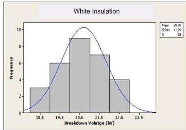
Figure 16 - Cable C breakdown voltage distribution
