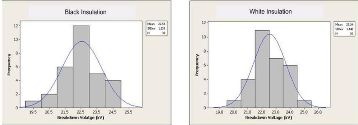
Figure 18 - Cable E breakdown voltage distribution
