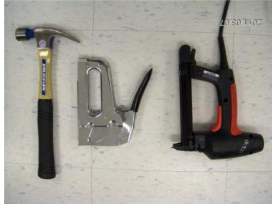
Figure 2 - NM cable installation tools
