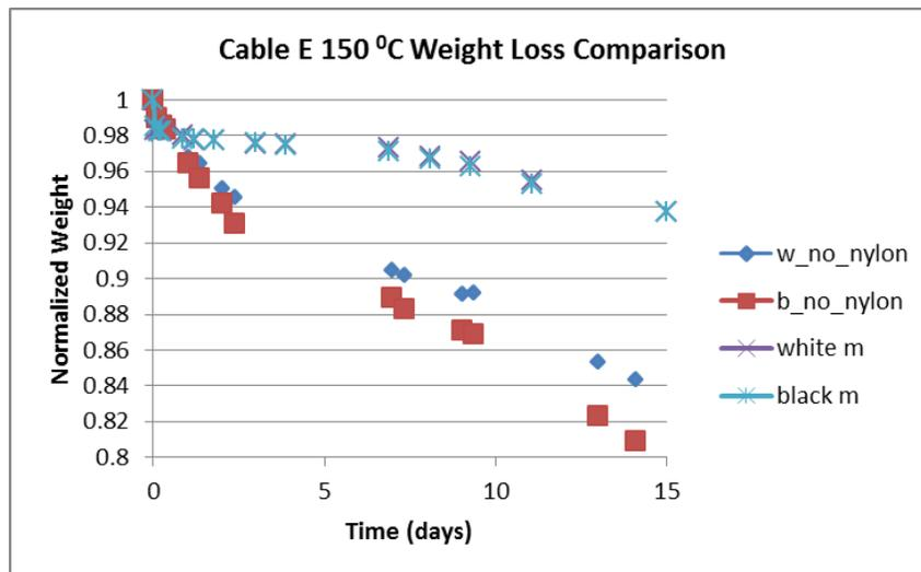
Figure 37– Comparison of Cable E insulation aging with and without nylon layer
