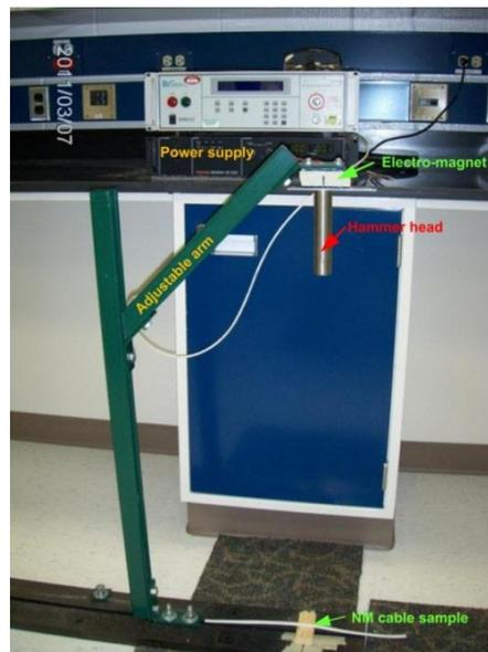
Figure 27 - Hammer impact simulator
