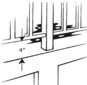
In addition, if an above-ground pool has a barrier on top of the pool, the **maximum vertical clearance between the top of the pool and bottom of the barrier should not exceed 4 inches**. Having these barriers for above-ground pools can prevent a child from climbing into them.
