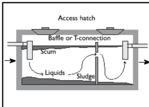
**Figure 4: Common Septic Tank (source: CMHC)**
